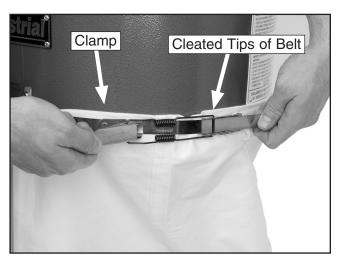
**Figure 12.** Securing collection bag onto collector.
